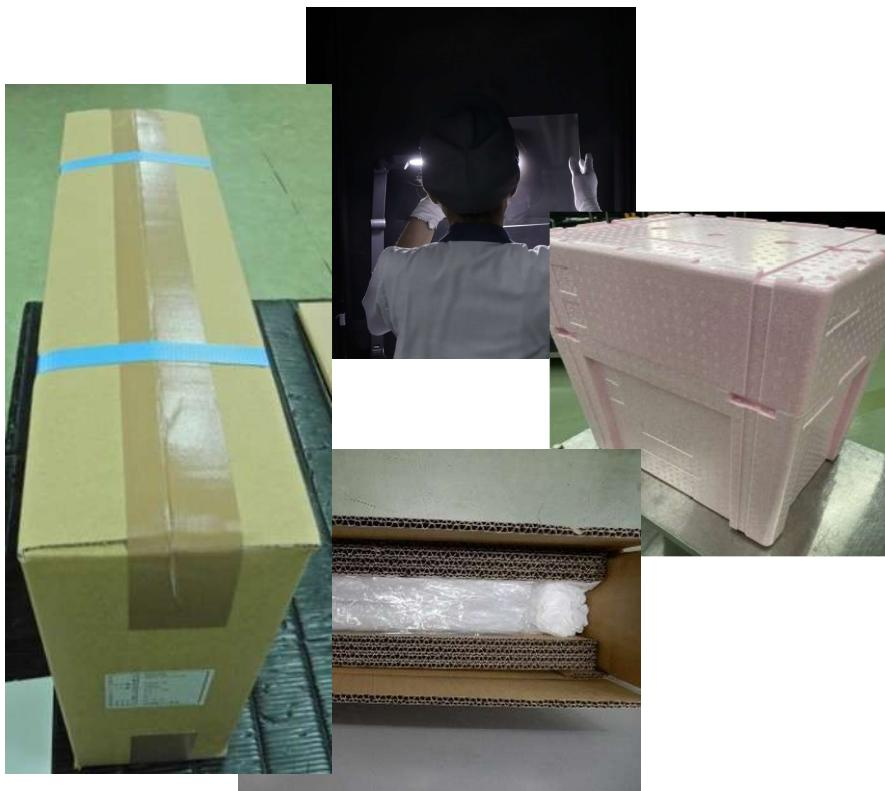
At Matsunami Glass Industry, we have established packaging specifications for various glass substrates. At Matsunami Glass Industry, we have established packaging specifications for various glass substrates. With inspections conducted in cleanrooms and careful selection of various cushioning materials and papers, we ensure safe and consistent delivery quality.
