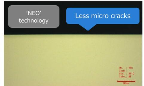
We can cut thinner glass like 0.03mm with NEO technology so as not to be broken easily if bent.
